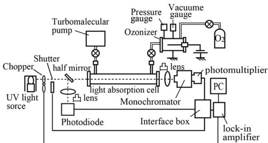
Fig.1: Experimental apparatus.
