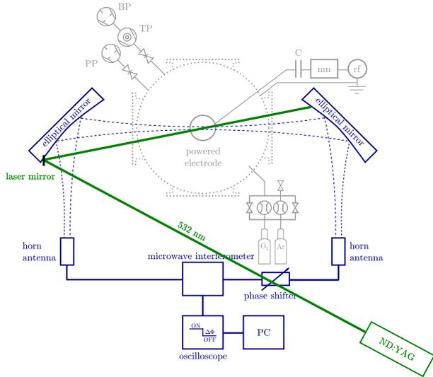
Fig. 1: Schematic top view picture of the discharge setup with the 160 GHz interferometer and the laser beam guidance of the Nd:YAG laser for photodetachment.
