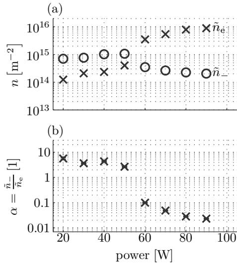
Fig. 2: (a) Mean on phase line integrated electron  $\tilde{n}_e$  (x) and negative ion density  $\tilde{n}_-$  (o) over rf power variation at 30 Pa and 5 sccm. (b) Is the electronegativity  $\tilde{n}_- / \tilde{n}_e$ .
