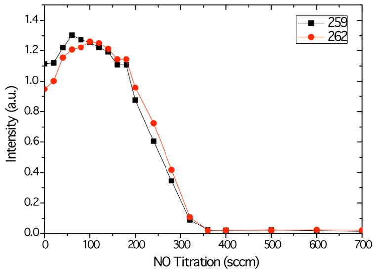
Fig.2 Intensities of NO $\beta$  ( 262 nm ) ( circles ) and NO $\gamma$  (259 nm)( squares) versus the Ar-1.5% NO flow rate introduced in the late afterglow after the pink (a) . N<sub>2</sub> gas with a purity of 99% at 1 slm , 8 Torr , 100 W.
