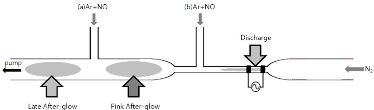
Fig. 1. Flowing afterglows in a downstream quartz tube of dia.21 mm after a capacitive RF discharge in an upstream tube of dia.6 mm and 30 cm length. An Ar-1.5% NO gas mixture can be injected after the early afterglow (a) or after the discharge end (b).
