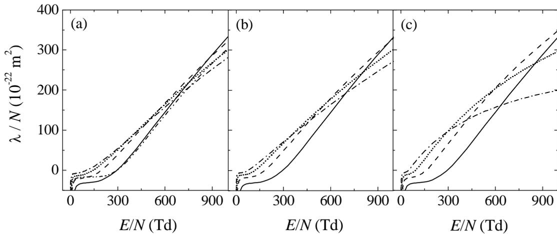
Fig. 1: Calculated  $\lambda/N$  as a function of  $E/N$  for mixtures of  $\text{Cl}_2$  with Kr (a), Ar (b) and He (c) for the following  $\text{Cl}_2$  percentages: 100% (solid line), 50% (dashed), 25% (dotted) and 10% (dashed-dotted). In (a) are presented calculations using [4] for pure  $\text{Cl}_2$  (dashed-dotted-dotted line).
