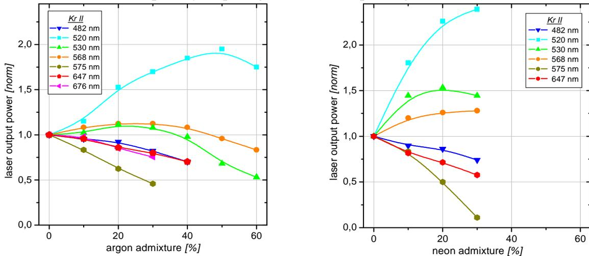
Fig. 1: Influence of argon (on left) and neon (on right) admixtures on laser power of krypton lines. Total gas pressure 200 mTr. Discharge current 40 A. Values normalised to values for pure krypton.
