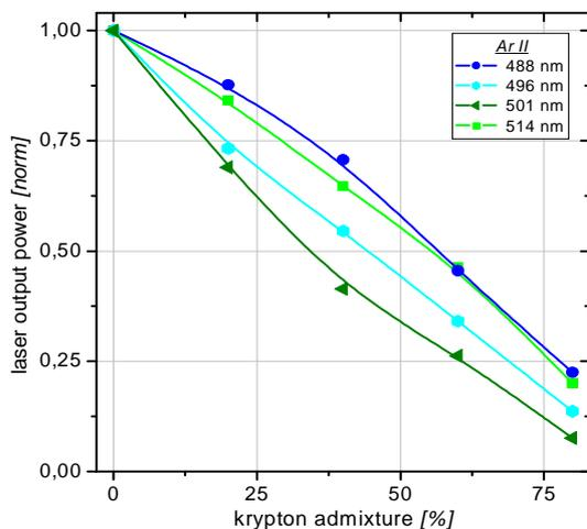
Fig. 2: Influence of krypton admixtures on laser power of exemplary argon lines. Total gas pressure 200 mTr. Discharge current 40 A.
