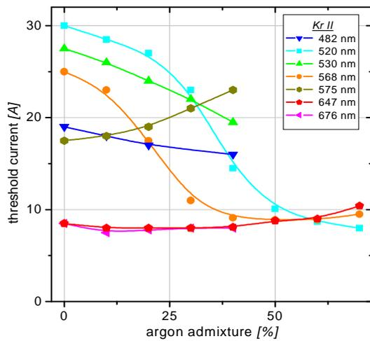
Fig. 3: Influence of argon admixtures on laser generation threshold current. Total gas pressure 200 mTr.
