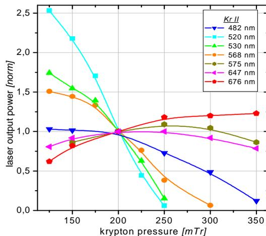
Fig. 4: Influence of krypton pressure on the power of krypton laser lines. Measurements was performed in pure krypton. 40 A discharge current.
