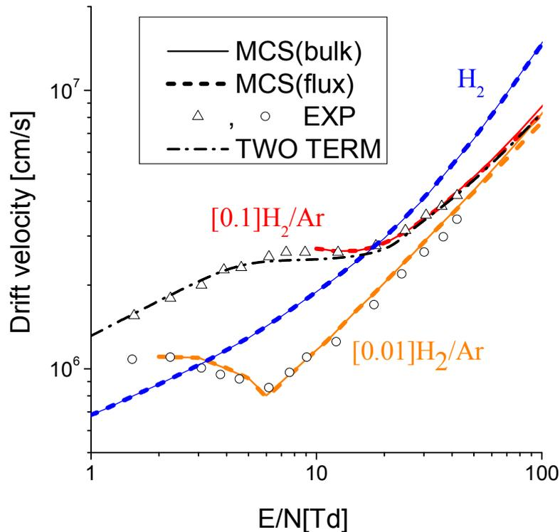
Fig. 1: Electron drift velocity for the mixture of Ar and H<sub>2</sub>.
