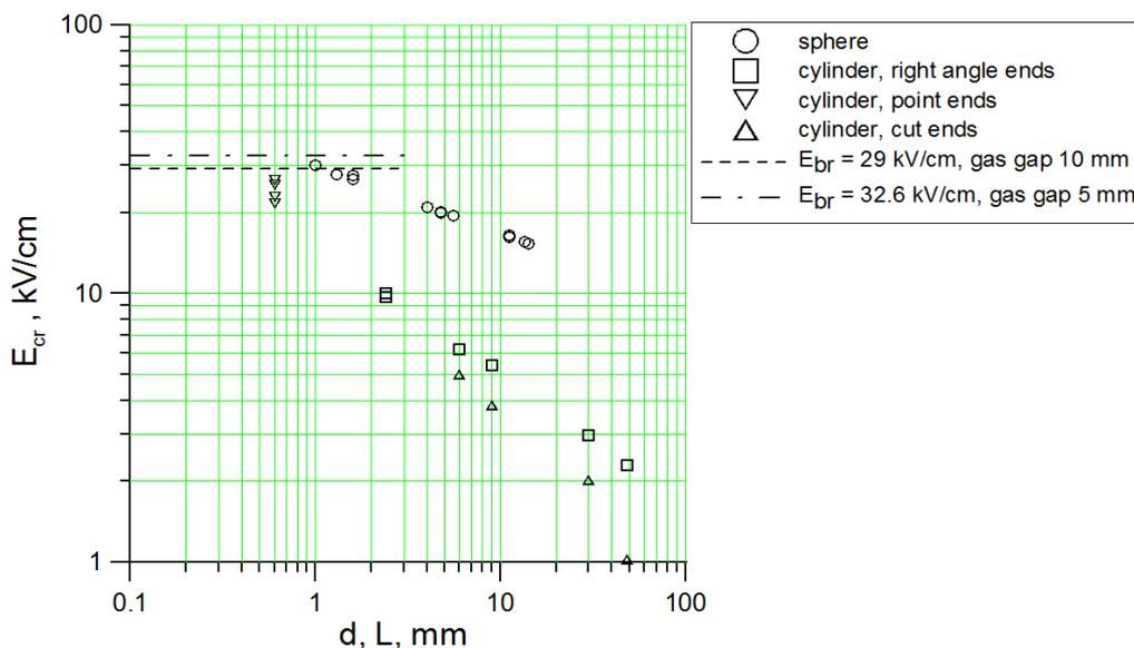
Figure: The dependence of discharge onset threshold electric field value  $E_{cr}$  on sphere diameter  $d$  and cylinder length  $L$ . The relation of  $L$  to cylinder diameter equals 30.
