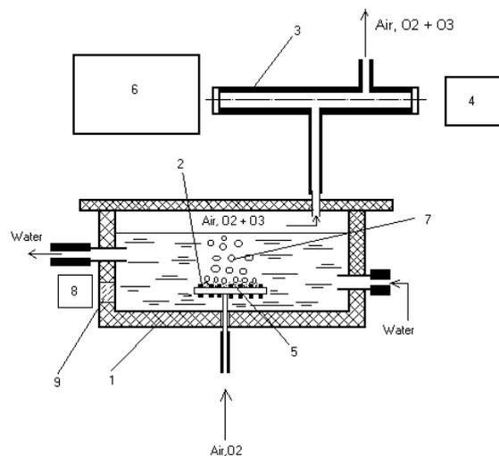
Fig. 2. Experimental layout. 1-vessel filled with water; 2-multi-spark discharger; 3-diagnostic quartz cell;4-deuterium lamp; 5-discharge plasma; 6-MDR-3 monochromator; 7-gas bubbles; 8-MUM-1 monochromator, and 9-quartz window.
