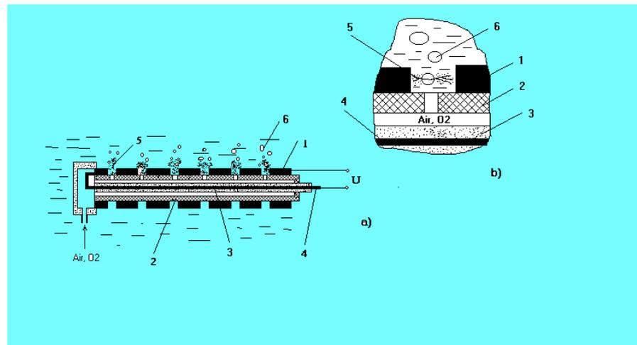
Fig. 1. Multi-electrode gliding surface discharge facility.
