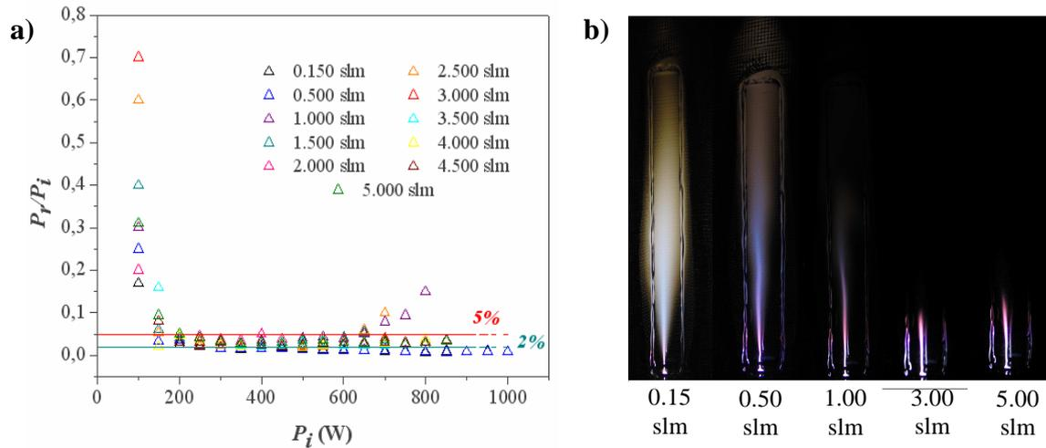
Fig. 1: a) Power reflection coefficient ( $P_r/P_i$ ) as function of power and gas flow rate, b) several images taken (1/250 exposition time) from the flame generated at 450 W with Ar flows of 0.15, 0.50, 1.00, 3.00 and 5.00 slm.
