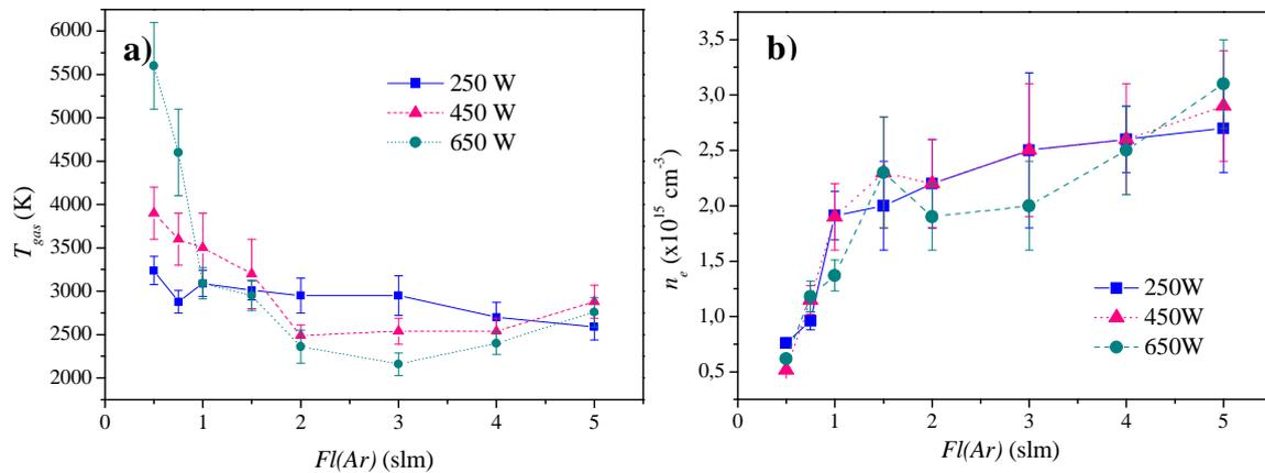
Fig. 2: a) Gas temperature obtained by means of the rotational temperature of  $N_2^+$  specie and b) electron density calculated from Stark broadening of  $H_\alpha$  line.
