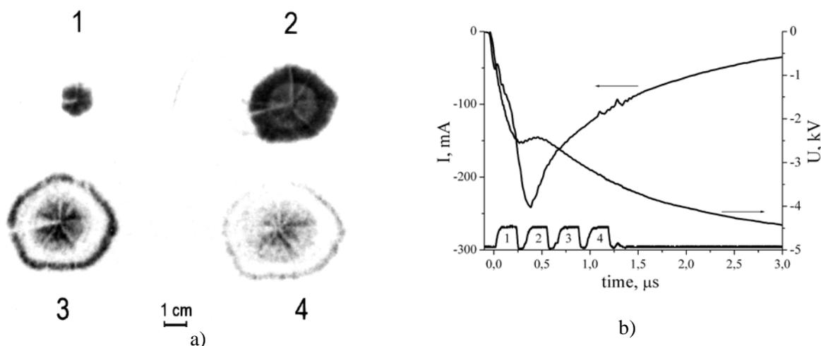
Fig. 1: **a)** The set of four successive instant images of plasma sheet in a pulsed pin-to-plane NSDBD in Ar at atmospheric pressure. Exposure time of each frame is 200 ns; time interval between neighbour frames is 100 ns; figures 1-4 numbering the frames in Fig.1a) correspond to those in Fig.1b); **b)** The current I and voltage U waveforms of the pulsed NSDBD; rectangular pulses (1-4) at the bottom of Fig.1b show a time position of the frames presented in Fig.1a.
