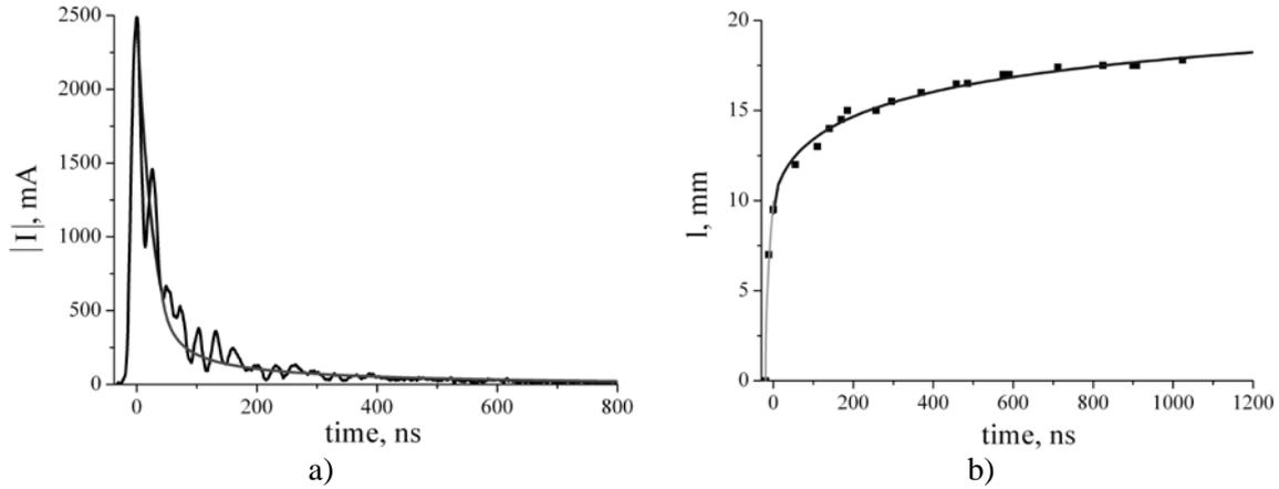
Fig. 2: a) the experimental (uneven curve) and calculated (even curve) waveform of current for pulsed NSDBD in air at pressure of 300 Torr; b) the dependence of of plasma sheet length  $l$  vs time (squares – experiment, smooth curve – theory).
