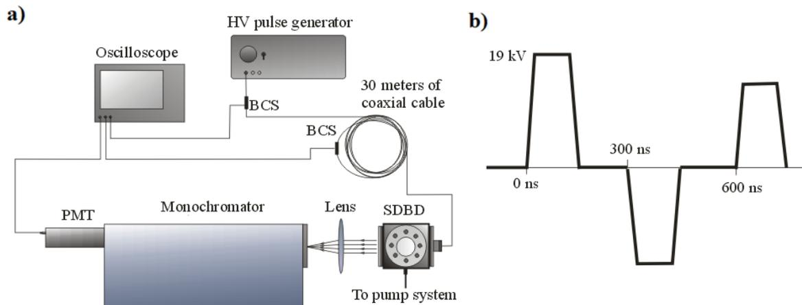
Fig. 1 (a): experimental setup. BCS – back current shunt. PMT – photomultiplier tube; (b): signal on the high-voltage electrode. First pulse – incident positive pulse, second and third – generator-reflected pulses.
