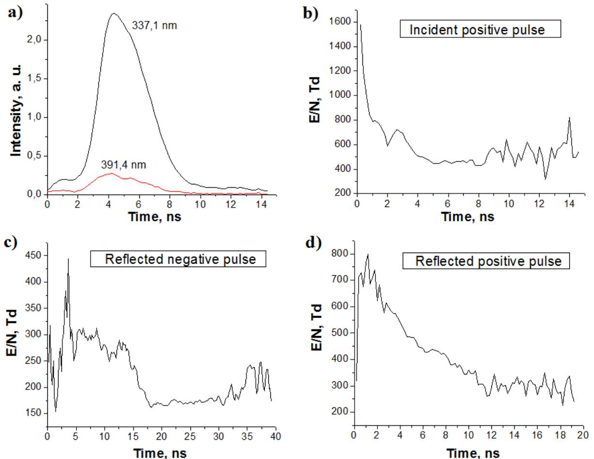
Fig. 2 (a): rate of intensities for wavelength of interests during incident positive pulse; (b): electric field evolution during incident positive pulse; (c): electric field evolution during negative reflected pulse; (d): electric field evolution during reflected positive pulse.
