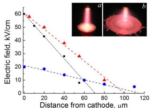
Fig. 1. Longitudinal electric field profiles for cooled (squares) and uncooled (triangles, circles) cathodes. Square and triangle symbols correspond to axial profiles, the circles – profile at a distance of 8 mm from the axis. The inset shows discharge photos with cooled (*a*) and uncooled (*b*) cathodes.
