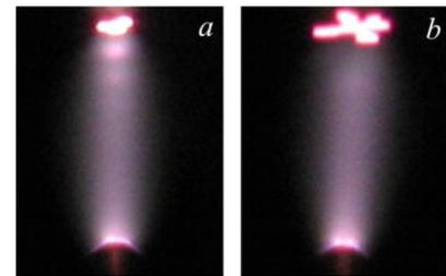
Fig. 2. Helium APGD images without (*a*) and with (*b*) additional cathode heating. Current is 0.05 A, gap is 10 mm. The cathode is on top.
