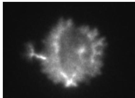
Fig. 7. Photo of the discharge forming streamer like structures propagating outside the bubble (nitrogen bubble volume 12  $\mu\text{l}$ , solution conductivity of 12.2  $\mu\text{S/cm}$ , applied voltage of 28 kV, recorded 60  $\mu\text{s}$  after HV application by exposure time of 5  $\mu\text{s}$ ). HV tip is at the bottom. Plasma volume is about 10x bigger with respect to Fig. 6.
