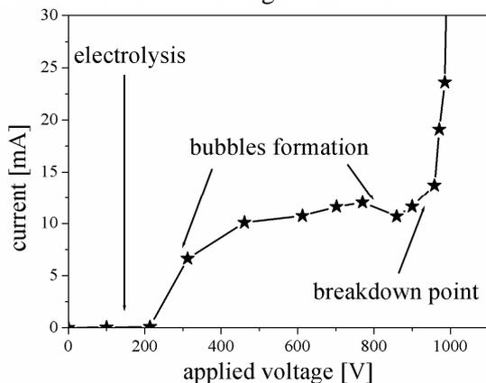
Fig. 2. Current-voltage characteristics of the pin-hole discharge with 0.4 mm barrier thickness.
