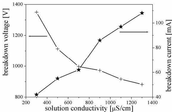
Fig. 4. Breakdown voltage and breakdown current as a function of the solution conductivity (pin-hole with diameter of 0.2 mm and thickness of 0.25 mm) [17].
