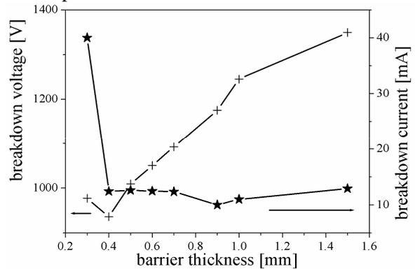
Fig. 5. Breakdown voltage and breakdown current as a function of the barrier thickness (solution conductivity of 460  $\mu\text{S/cm}$ ).
