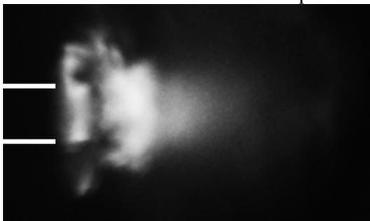
Fig 6. Photo of the discharge forming streamer like structures propagating outside the bubble (barrier thickness of 1.5 mm, applied voltage 1.6 kV, discharge current 300 mA, exposure time of 1 ms). Capillary is marked by white lines.
