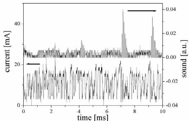
Fig. 3. Current and sound records during the bubbles formation (barrier thickness of 0.4 mm, applied voltage of 620 V).
