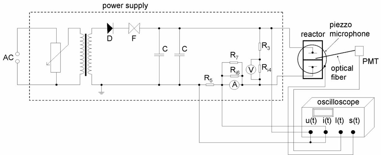
Fig. 1: Full scheme of the experimental setup used for the presented observations; D – HVR-1x7 SB 3714, F – safety-fuse 0.5 A, C – 0.85 μF microwave capacitor 25M854S095T, 2500 VA, R3 – 100 MΩ, R<sub>14</sub> – 3.114 kΩ, R<sub>5</sub> – 5.13 Ω, R<sub>16</sub> – 105.5 Ω, R<sub>7</sub> – 0.13 Ω.
