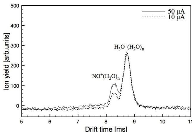
Fig. 1: IMS spectrum of NO<sup>+</sup>(H<sub>2</sub>O)<sub>n</sub> and H<sub>3</sub>O<sup>+</sup>(H<sub>2</sub>O)<sub>n</sub> reactant ions for different CD current
