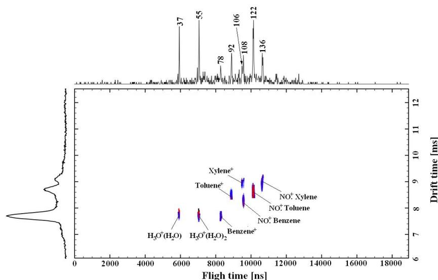
Fig. 2: 2D IMS/MS map of BTX molecular and  $\text{NO}^+$  adducts ions measured in zero air.
