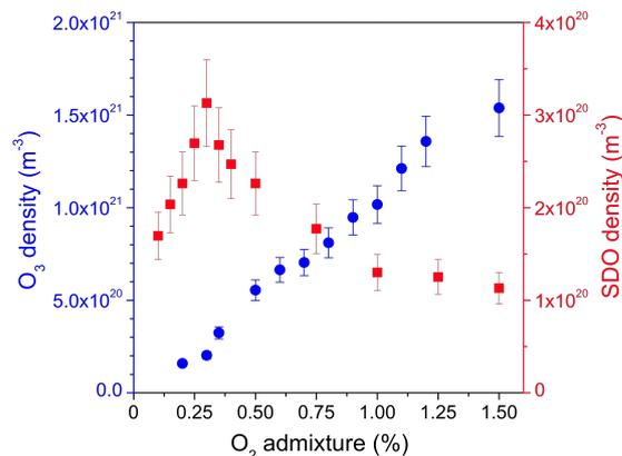
Fig. 3:  $O_2(a^1\Delta_g)$  and  $O_3$  densities as a function of the molecular oxygen fraction in the gas mixture (He/ $O_2$ ). Plasma jet (kHz-APPJ) operation at 6 kV and 20 kHz, with a He flow of 2 slm.
