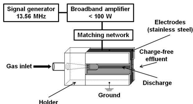
Fig. 2: Schematic of the RF-driven atmospheric pressure plasma jet.
