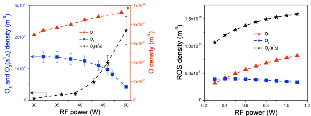
Fig. 4: Measured (left) and simulated (right) ROS densities as a function of RF generator power. Plasma jet (RF-APPJ) operation with a He flow of 1 slm, and 0.5% of  $O_2$  admixture.
