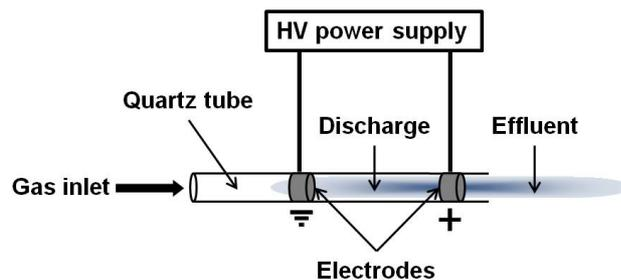
Fig. 1: Schematic of the kHz-driven atmospheric pressure plasma jet.
