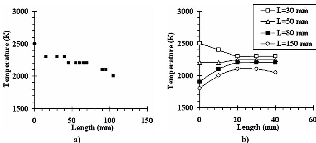
Fig. 2: Axial distribution of temperature in flame: (a) – without combustion chamber; (b) – outlet of combustion chamber.
