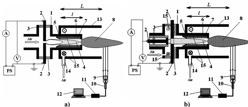
Fig. 1: The schematic view of the plasma-dynamic system (PDS) for combustion activation of the paraffin containing solid mixture with transversal (a) and rotating gliding arc (b).
