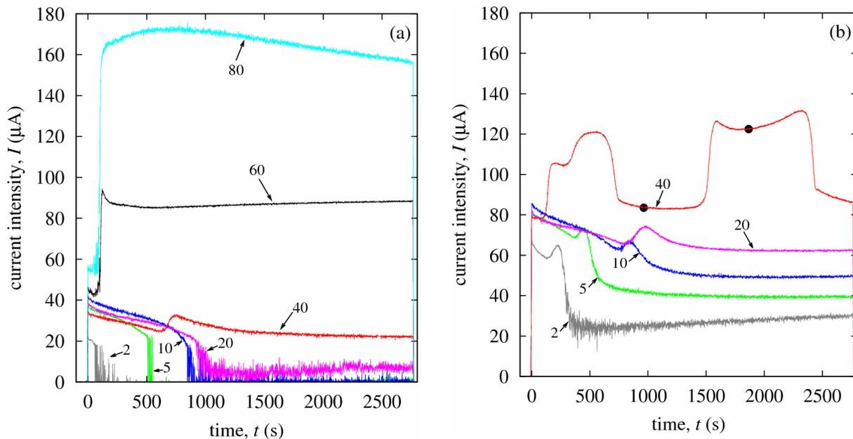
Fig. 1: Time evolution of corona current intensity in mixtures of CO<sub>2</sub> and N<sub>2</sub> for (a)  $V = 7$  kV and (b)  $V = 8$  kV. The volume percentage of N<sub>2</sub> corresponding to each line is indicated in the figure.
