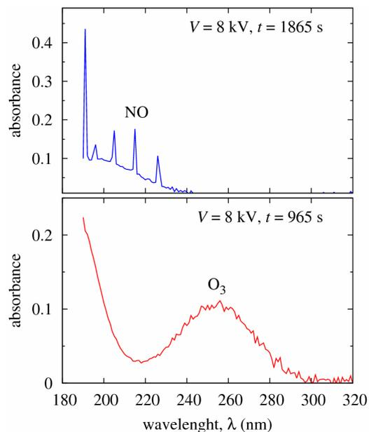
Fig. 3: UV spectra of a gas mixture of 40% N<sub>2</sub> and 60% CO<sub>2</sub> for an applied voltage  $V = 8$  kV and at two different times: 1865 s (top) and 965 s (bottom). These times are indicated with a black dot in Fig. 1.
