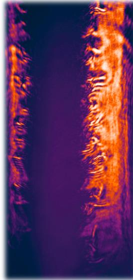
Figure 2. Laser shadowgram of MRT in ablated foil plasma ( $\sim 200$  ns).
