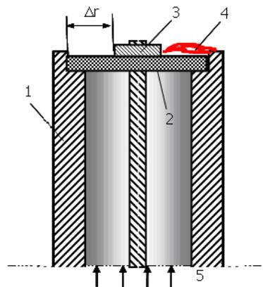
Fig. 1. Scheme of “Microwave Arc”. 1-outer electrode; 2-quartz disk; 3-inner electrode; 4-discharge channels; 5-microwave radiation.
