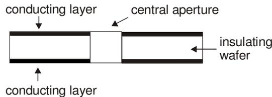
Discharges were generated in a range of gases, and device operation was characterized by electrical and optical measurements. Breakdown voltages of 300-500 V and discharge currents of 0.1-2 mA were measured for different operating conditions. Preliminary measurements of Paschen curves for these devices indicated a minimum breakdown voltage in the region of 2-5 Torr cm, as expected for glwo discharges. Device lifetimes appear to be in excess of many tens of hours.
