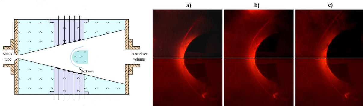
Fig. 1: Setup scheme. Schlieren flow pictures with different incoming flow parameters.
