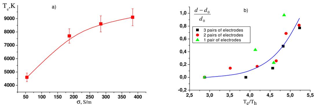
Fig. 2: a) Electron temperature vs plasma conductivity at gas discharge current increase.
