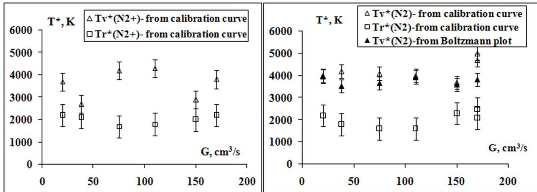
Fig. 1 Dependence of the vibration and rotation temperatures of  $N_2$  molecule and of molecular ion  $N_2^+$  in TA plasma on the gas flow rate  $G$ .
