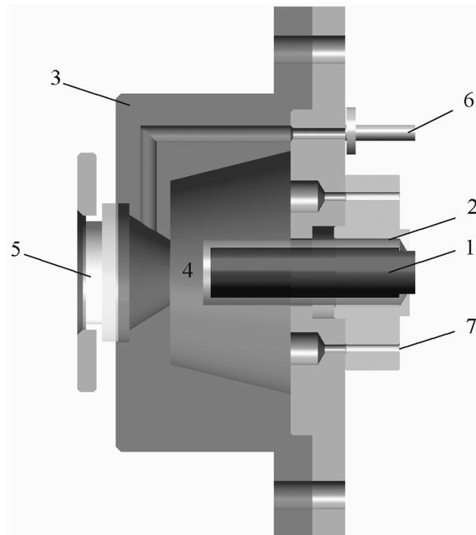
Fig. 1: Scheme of one barrier flow Ar<sub>2</sub>-excilamp. 1 – high voltage electrode, 2 – quartz tube, 3 – metal case, 4 – discharge gap, 5 – LiF output window, 6 – gas inlet, 7 – gas outlet
