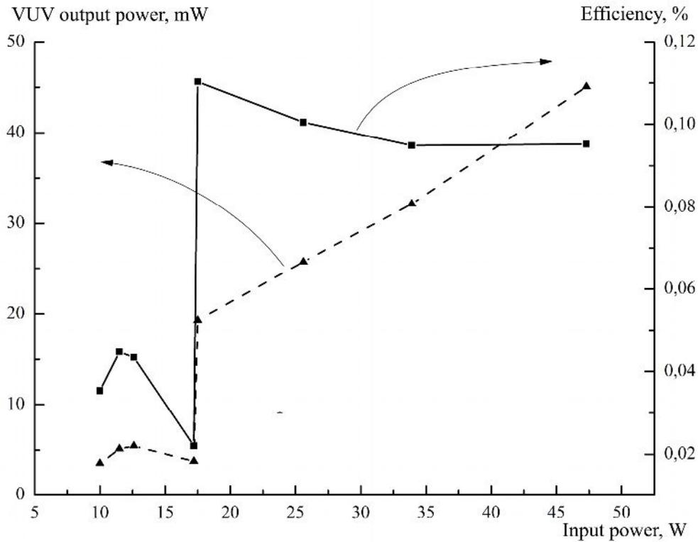
Fig. 2: VUV output power and efficiency of radiation versus input power
