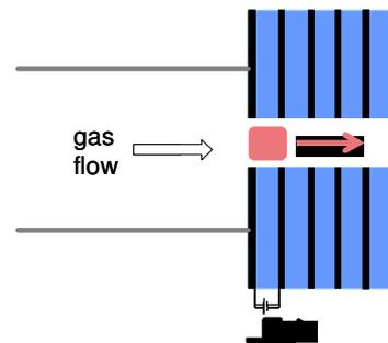
Fig. 1: Geometry of the multi-electrode microplasma device.
