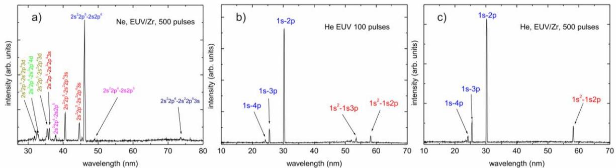
Fig. 2: Spectra of Ne and He gases ionized with EUV radiation pulses with and without Zr filter: a) Ne gas irradiated through Zr filter, b) He gas irradiated with no filter, c) He gas irradiated through Zr filter
