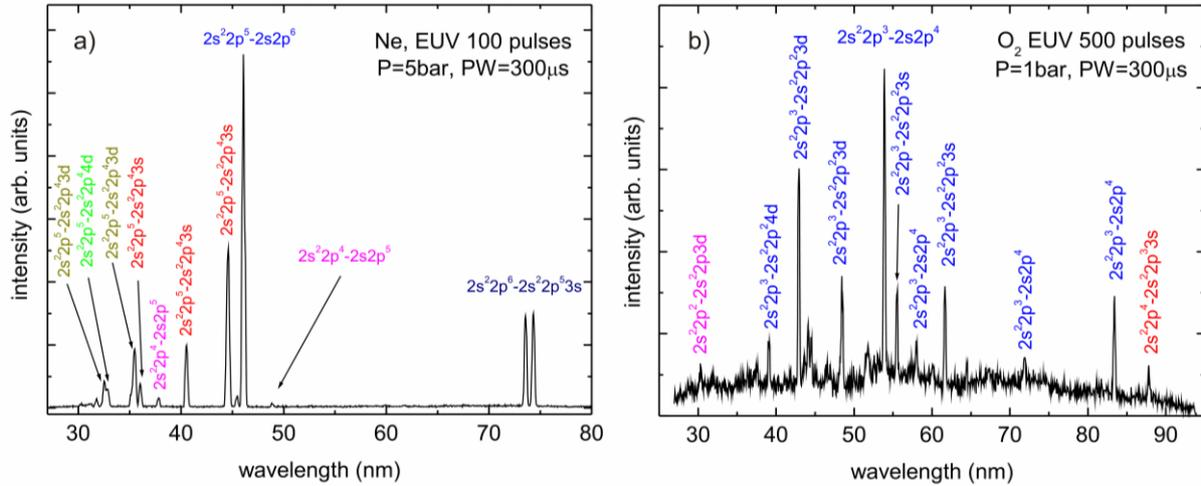
Fig. 1: Spectra of gases ionized with EUV radiation pulses from a laser-plasma source: a) neon, b) oxygen
