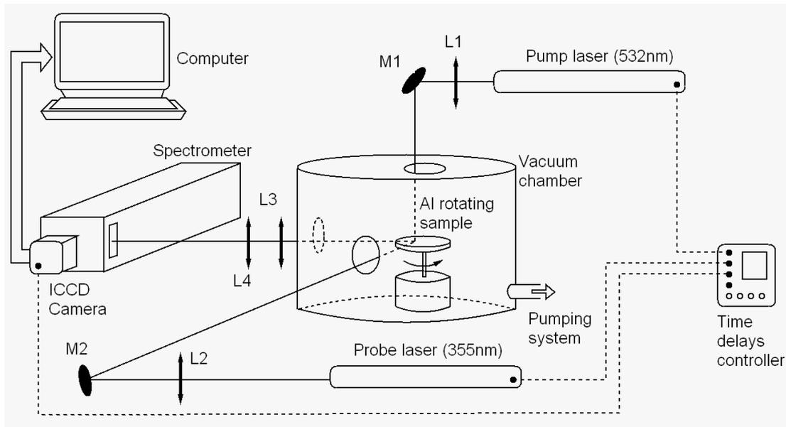
**Fig.1.** Thomson Scattering setup for LIBS experiments performed in vacuum.
