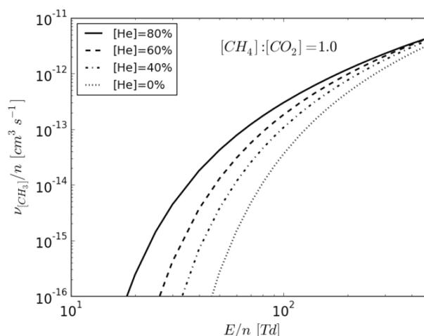
Fig. 1: Variation of the density-normalized collision frequency for dissociation of CH<sub>4</sub> into CH<sub>3</sub> as a function of the reduced electric field, in mixtures with different concentration of helium.
