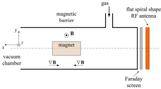
Fig. 2 Layout of the quartz tube with the magnetic field, the planar RF antenna and the Faraday shield.
