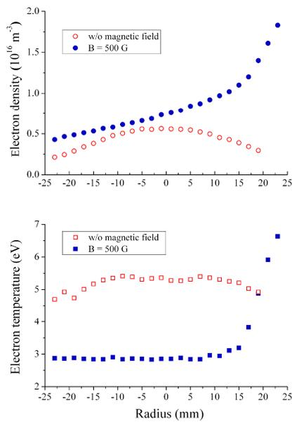
Fig. 3 Radial distribution of  $n_e$  and  $T_e$  in Ar at the tube outlet with magnetic field and strip formation and without a magnetic field.
