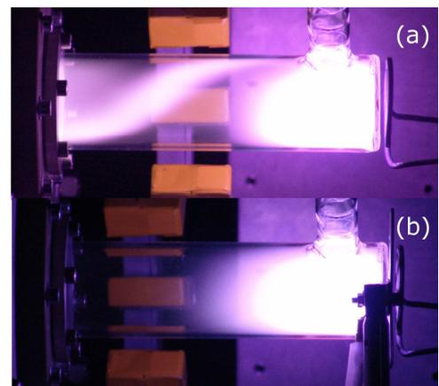
Fig. 1 Pictures of the RF discharge with 20 sccm argon, 300 W input power, at a background pressure of around  $10^{-3}$  mbar and 500 G magnetic field without (a) and with (b) a Faraday shield. The strip is clearly visible in case (a).
