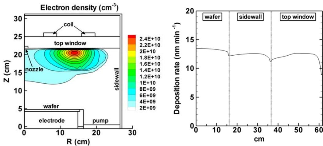
Fig 1. (Left) 2D reactor geometry and electron density profile and (right) the calculated  $\text{SiO}_2$  deposition rate.
