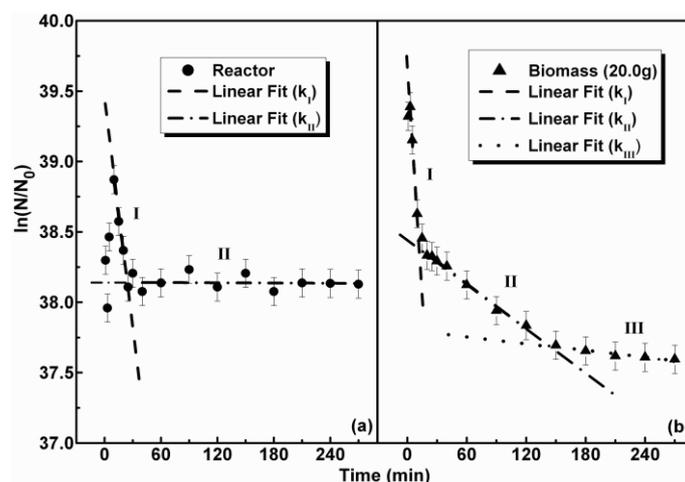
Fig. 1. Ozone decomposition as a function of time: (a) stainless steel reactor wall (circles) and (b) bagasse surface (triangles).
