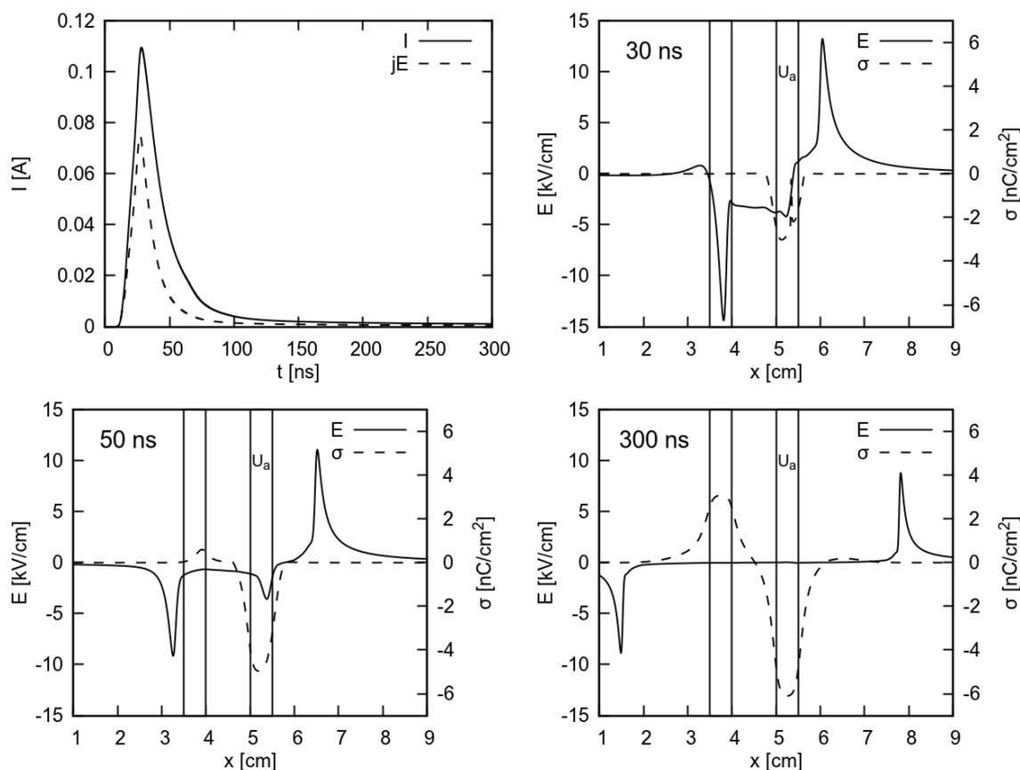
Fig. 1: The discharge current and current due to Joule heating are shown on left top figure. Other figures show the electric field on axis of symmetry and surface charge density on tube interface for times  $t = 30, 50$  and  $300$  ns. The grounded ring is shown as rectangle with label  $U_a$  between 5 and 5.5 cm.  $U_a = 12$  kV.
