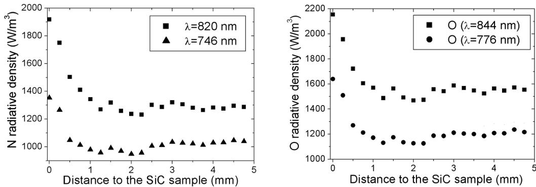
Fig. 2: Radiative density of N (left) and O (right) near infrared lines on the axis of the plasma flow within the boundary layer in front of the SiC sample
