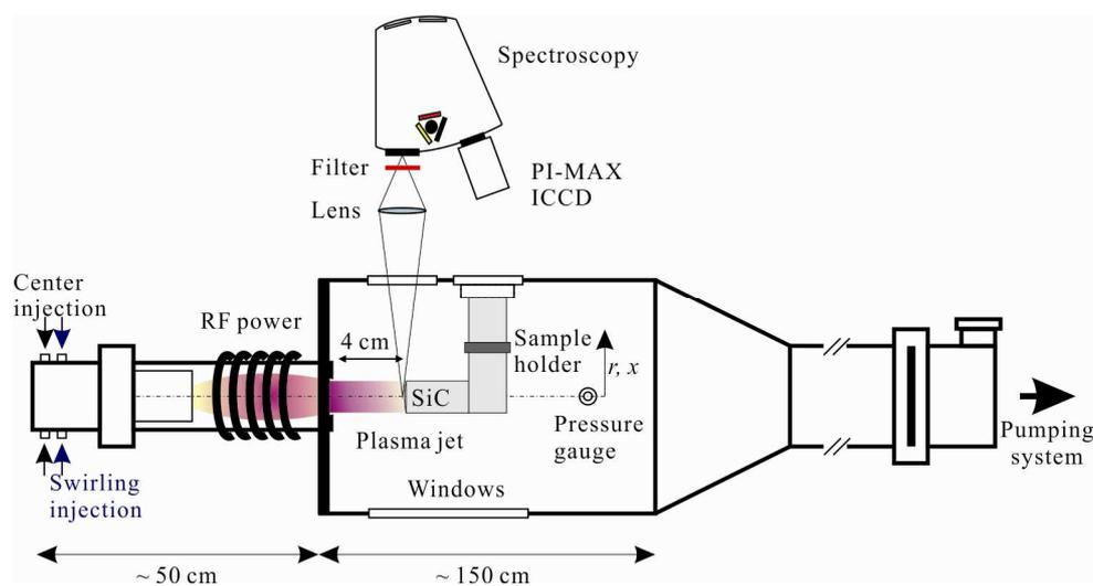
Fig. 1: Overview of the plasma wind tunnel, the SiC sample and the emission spectroscopy setup.
