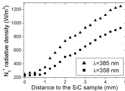
Fig. 3: Radiative density of  $N_2^+$  first negative system on the axis of the plasma flow within the boundary layer in front of the SiC sample
