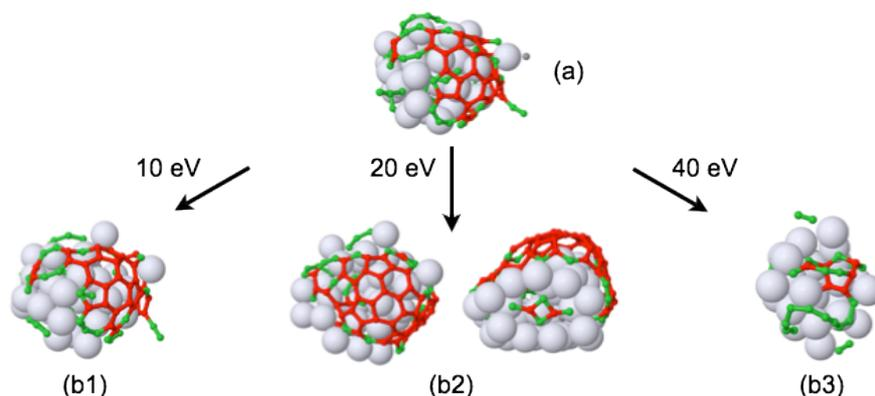
Fig. 2: Effect of Ar ion bombardment energy on the carbon network. (b1) At low energy, no effect is observed. (b2) At intermediate energy, the network is enhanced. (b3) At high energy, the network is destroyed.
