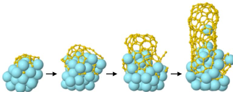
Fig. 1: Evolution of a vertically growing SWNT on a Ni-nanocluster, in alignment with an applied E-field.
