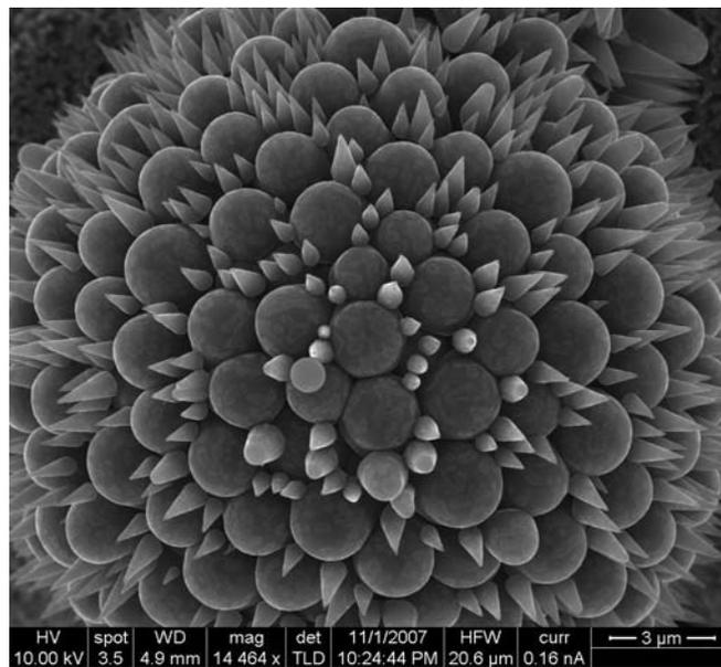
Fig. 2: SEM image of a reshaped carbon structures with the CH<sub>4</sub> plasma and Boron atoms.
