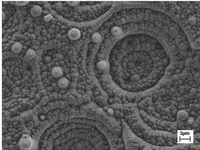
Fig. 1: SEM image of HOPG graphite surface after interaction with oxygen plasma species in weakly ionised highly dissociated plasma.
