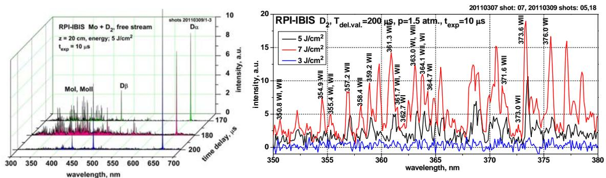
Fig. 3. Optical spectra of free plasma streams in RPI-IBIS at different  $\tau$  values (left) and a part of the spectrum of plasma produced from the W-target at different flux densities (right).
