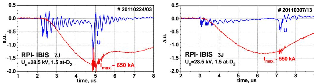
Fig. 2. Current- and voltage-waveforms recorded at plasma flux density equal to  $7 \text{ J/cm}^2$  and  $3 \text{ J/cm}^2$ .
