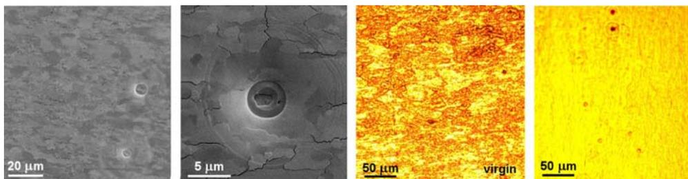
Fig. 4 SEM (left) and optical microscope (right) images of the W-target surface before (virgin) and after its irradiation by the pulsed deuterium-plasma stream ( $7 \text{ J/cm}^2$ ) in the RPI-IBIS facility.
