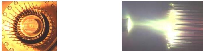
Fig.1. End-on view of the RPI-IBIS electrodes (left) and the side-on picture of the visible radiation from a deuterium-plasma stream interacting with the W-target (right).
