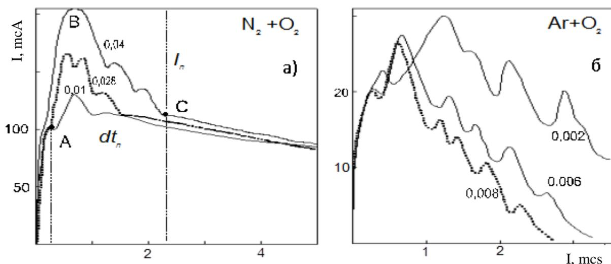
Fig.1. Typical forms of the measured corona current pulses: a) in nitrogen, б) in argon with the admixture of oxygen at concentrations %, marked by numbers
