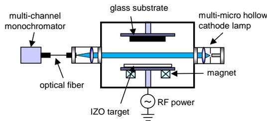
Fig. 1 Experimental set-up of magnetron sputtering reactor and the optical system of absorption spectroscopy employing the multi-MHCL.
