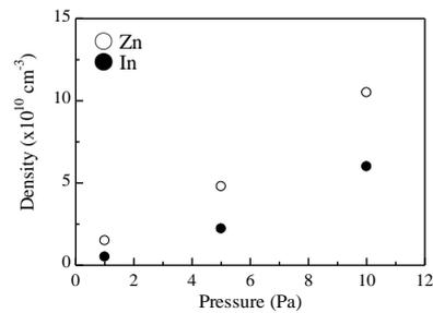
Fig. 2 Absolute densities of Zn and In atoms as a function of pressure.
