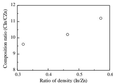
Fig. 3 Concentration ratio of In to Zn content in the IZO films ( $C_{\text{In}}/C_{\text{Zn}}$ ) as a function of In/Zn density ratio.
