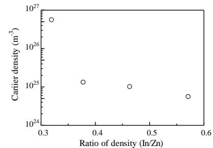
Fig. 4 Carrier density as a function of In/Zn density ratio.
