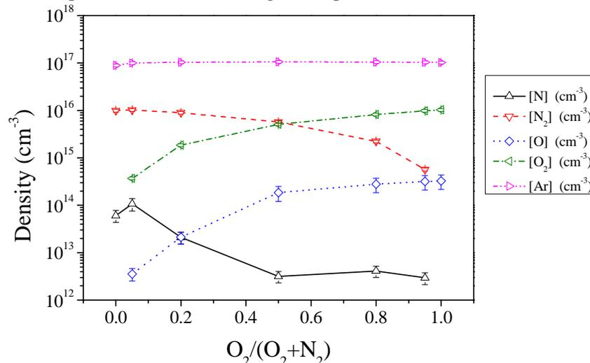
Fig. 2 : Species density vs gas composition in a 180 sccm Ar, 20 sccm O<sub>2</sub>+N<sub>2</sub> for different O<sub>2</sub>/(O<sub>2</sub>+N<sub>2</sub>) ratios at 100 W microwave power, 5.6 mbar pressure and 345 K gas temperature.
