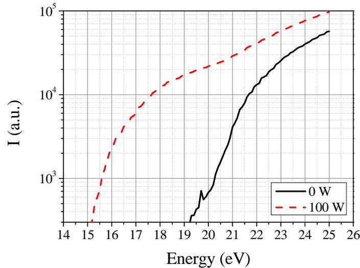
Fig. 1 : Mass spectrometry signal intensity in RGA mode at  $m/z = 16$  as a function of electron energy for plasma on and plasma off conditions in Ar/O<sub>2</sub> gas mixture (70 sccm, 7.8 sccm, 100 W, 3.7 mbar)
