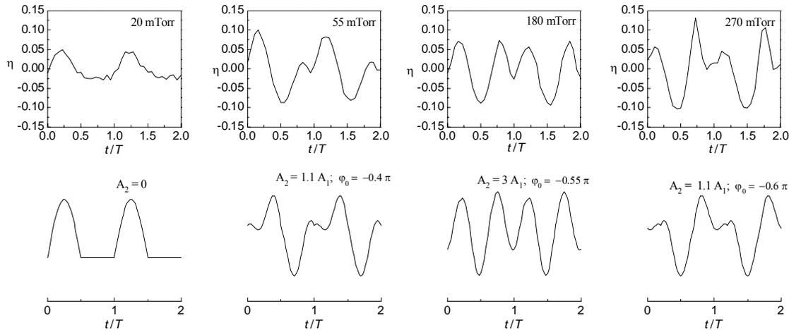
Fig. 1. First row: Time variation of the measured normalized intensity  $\eta$  at a given point during two rf cycles of the signal sustaining the discharge. Second row: The sum of the functions  $f_1$  and  $f_2$ . The values of the parameters (amplitude and initial phase) chosen give the best fit to the results from the measurements. Applied power 100 W at 27 MHz.
