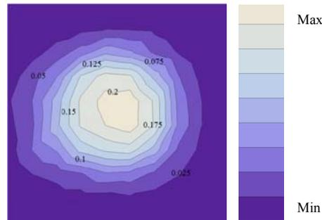
Fig. 2. Spatial distribution over the discharge cross section of the second harmonic of  $\eta$  and, respectively, of the squared rf electric field intensity (arbitrary units) at 100 W and 180 mTorr.
