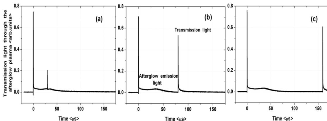
**Figure 1** The temporal profile with long afterglow of the Ne 588.1 nm emission line and the transmission light of the spectral lamp synchronized with the pulsed discharge and positioned at various temporal position in the afterglow; (a) 30 $\mu\text{s}$ , (b) 80 $\mu\text{s}$  and (c) 165 $\mu\text{s}$
