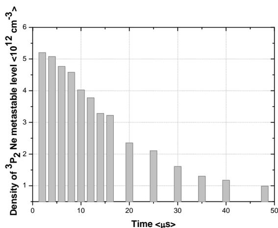
**Figure 3.** The temporal evolution of  $^3\text{P}_2$  Neon metastable level concentration during the hollow cathode afterglow plasma according to the absorption measurements on 588.1 nm transition
