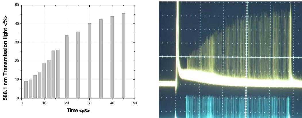
**Figure 2.** Temporal evolutions of the transmission signal of the 588.1 nm line of Neon; (a) calculated; (b) experimental (the trigger signal at the bottom)
