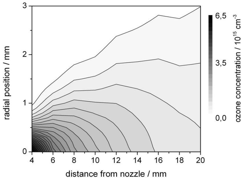
Fig. 2: Map of the space resolved ozone density distribution. The plasma jet nozzle is located at 0 mm distance from nozzle [1].
