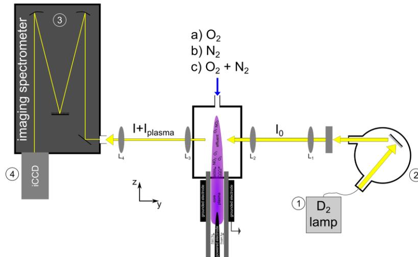
Fig. 1: Schematic setup of the ozone measurements with the deuterium lamp (1), a UV sensitive monochromator (2), an imaging spectrometer (3) and an iCCD detector.
