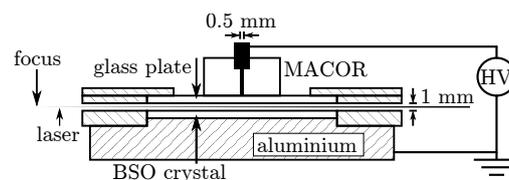
Fig. 1: Cross section of the discharge cell along the laser axis. The laser diverges in the gap due to its focus in front of the discharge cell.
