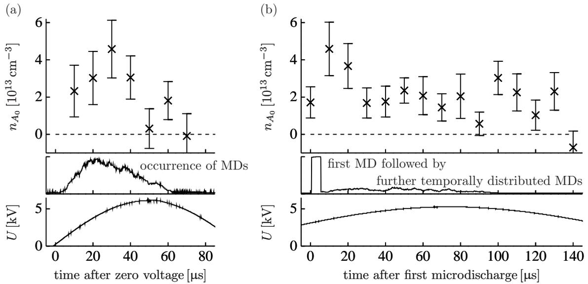
Fig. 2: Density of metastable  $N_2(A^3\Sigma_u^+, v=0)$  molecule in front of the glass plate (=anode) depending on time (a) in the positive half cycle (500 mbar, 5 kHz, 12.5 kV<sub>pp</sub>) and (b) after the first microdischarge (500 mbar, 2 kHz, 10.5 kV<sub>pp</sub>).
