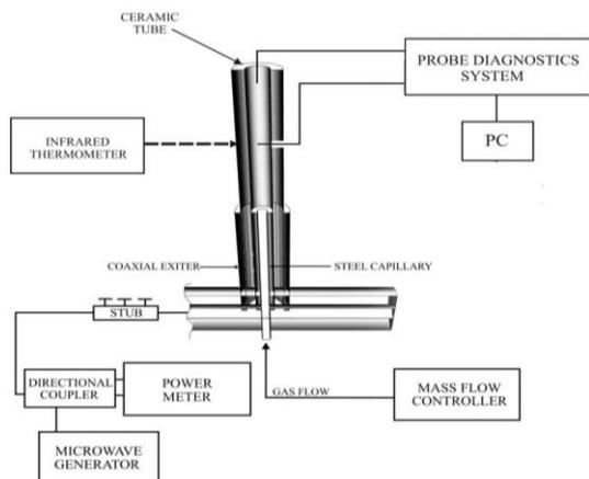
Fig. 1: Experimental setup with double probe.
