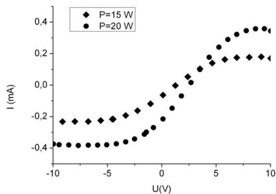
Fig. 2: Double probe characteristics.
