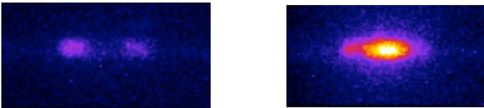
Fig. 2: Left: ICCD image taken with the laser tuned 0.0075 nm off resonance. The observed light is due to scatter of the laser from the windows of the plasma jet, leaking through the interference filter. Right: ICCD image taken with the same settings but with the laser tuned to the 2-photon excitation at 206.6505 nm.
