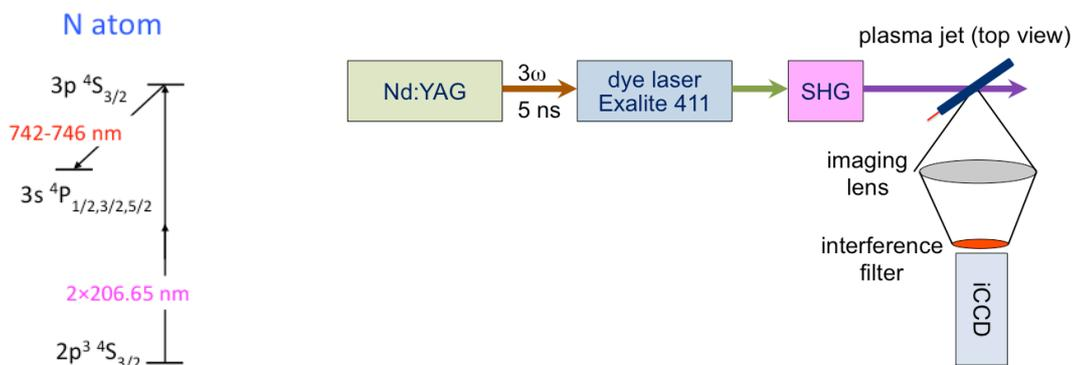
Fig. 1: Left: Excitation scheme for TALIF measurements on atomic nitrogen. Right: Experimental arrangement for TALIF measurements.
