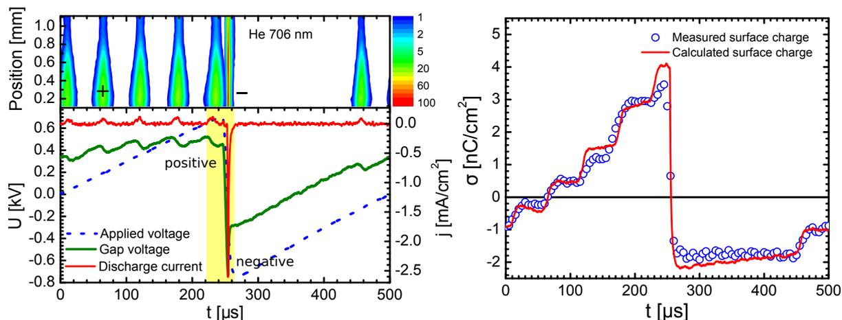
Fig. 1: Sawtooth voltage signal induces the Townsend-like mode and the glow-like mode in one period. Left: Combination of cross-correlation spectroscopy (He :706nm) with the electrical measurements. Right: Correlation of deposited surface charges with transferred charges.
