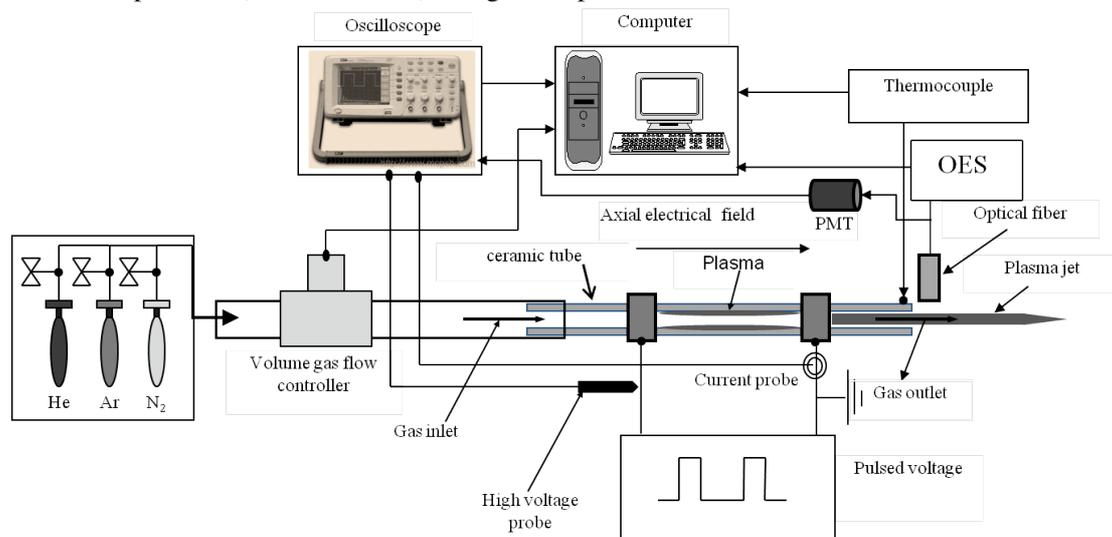
Fig. 1: Experimental setup of DBD-based plasma jet.
