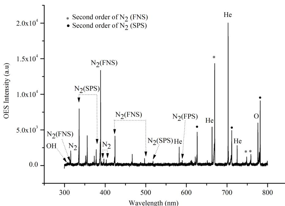
Fig. 2: Optical emission spectrum of the plasma jet flowing out into the environmental air (Helium flow rate = 3slm,  $V = 6\text{kV}$ ,  $\nu = 15\text{kHz}$ , duty cycle = 2%).
