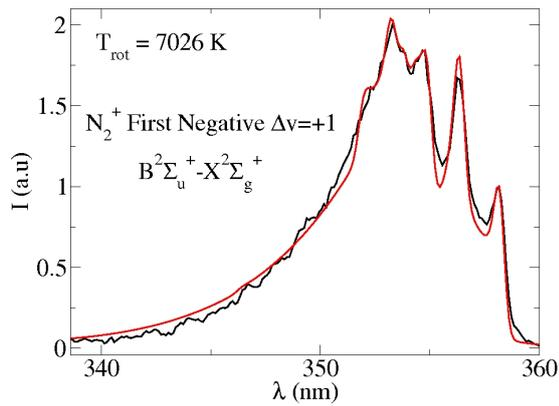
(a) Best fit obtained in the first expansion zone at 25 mm from the throat ( $r = 17$  mm).
