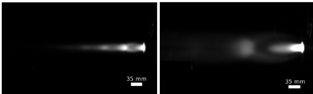
Fig. 1: Underexpanded (left) and highly underexpanded (right) supersonic air plasma jets.
