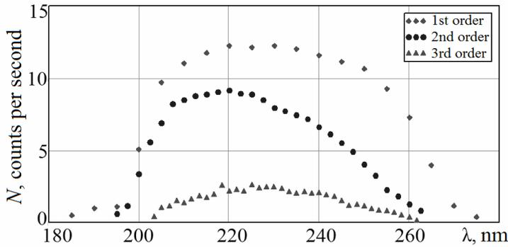
Fig. 2. Spectral dependencies of the photoreceptor's response (counts per second) to the radiation of the argon RF plasma for three diffraction orders: upper line – first order, middle line – second order, lower line – third order.
