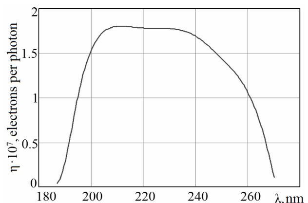
Fig. 1. Quantum response of the gas-filled photoreceptor with copper cathode.
