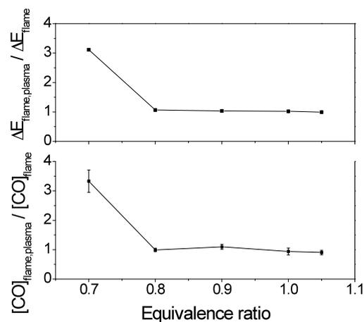
Fig. 1: CO density measurements in confined system function of ER with or without plasma. Fig. 2: CO density ratio (bottom) and gas kinetic energy ratio (top) with and without plasma function of ER.
