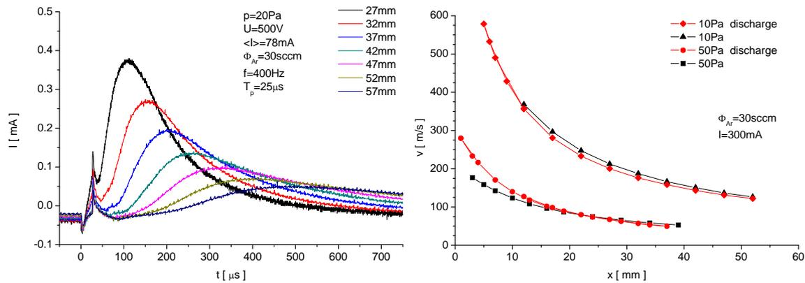
Fig. 2. Left graph: Typical course of the ion current to the negatively biased probe for different distances between the probe and the nozzle. Right graph: Comparison of results obtained from Pitot tube measurements on dependence whether the discharge is on or off.
