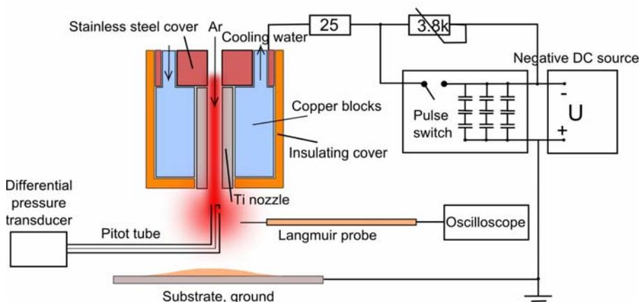
Fig. 1. Scheme of the low pressure hollow cathode plasma jet sputtering system with the Pitot tube and Langmuir probe used for the flow velocity measurements and the power supply circuit for the pulse excitation of the discharge.
